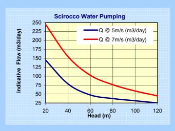
In run-of-the-wind water pumping applications, the Scirocco WT sets new standards by its direct electrical pumping concept coupled to Maximal Power Point Tracking controlled pump motor drive.
