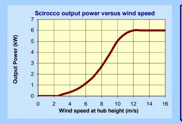
The Scirocco wind turbine is characterised by a very high efficiency in the lower to medium wind speed range which is prevailing most of the time (>80%). This is achieved through the combination of an optimised 2 blade rotor, efficient direct drive PM generator and maximum power point tracking control following the constantly varying wind speed.
