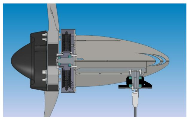
The LE-3000 is precision engineered in the UK with only two moving parts so little maintenance is required during the turbine's long operating life.
