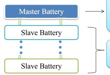
Master battery's sleep condition (US2000B and US2000 Plus): all slave batteries are turned off or slept. In this reason US2000 Plus battery as a master battery, it will act just same as a US2000B.
