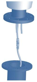
Using **three electrical connectors** joint the cables coming from the slip rings with the cables going down the tower.
