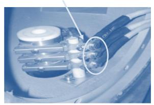
Check the spring tension, the correct connection of the brushes with the rings and the wire connections. Clean the set if necessary. In case the set is not in good condition replace the brushes. (See point 9 of this section, "Replacing the brushes").
