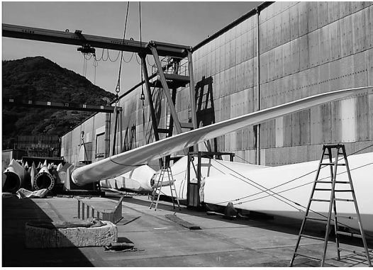
Fig. 16 Maximum load test of 36 m blade for 2 000 kW
