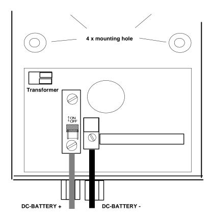
Take care of correct grounding of the inverter and your equipment that is connected to the inverter! We recommend to use an earth cable with minimum cross section of  $10 \text{mm}^2$  to ground the inverter. This will help to protect your unit in case of lightning. Be sure to meet all regulations about lightning protection!
