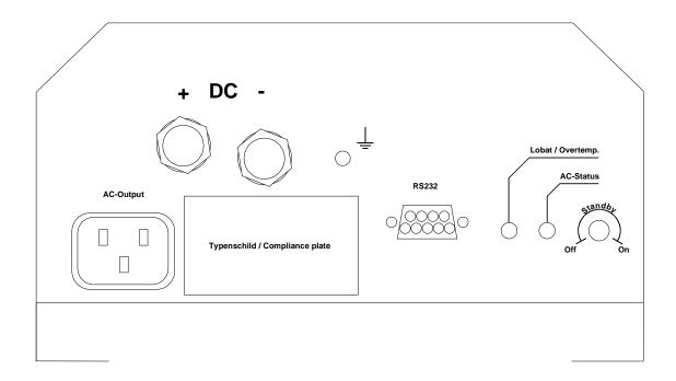
LED LOBAT: Battery voltage low. The inverter switches off automatically if
