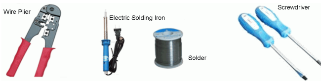
Figure 5.25 Tools for Making a Communication Cable
