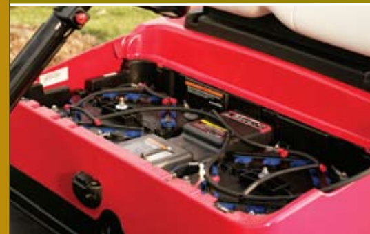
single-point watering system
