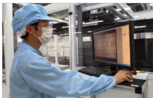
One hundred per cent micro-optical electroluminescent inspection
