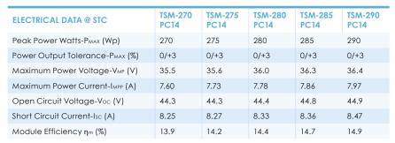
Values at Standard Test Conditions STC (Air Mass AM1.5, Irradiance 1000W/m², Cell Temperature 25°C).
