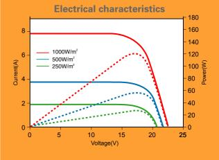
At STC( Standard Test Conditions).1000W/m<sup>2</sup>, 25°C cell temperature, AM1.5 spectrum
