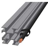
Fig. 10: Fixing the cable at A2 mounting rail with PV-clamp
