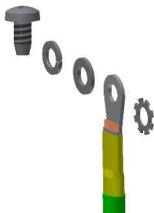
Fig.18:grounding set for the frame
